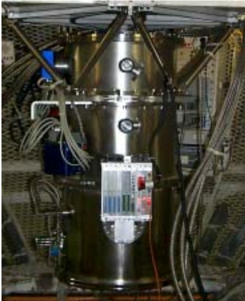
IRIS 2 mounted at the Cassegrain focus of the 3.92-m Anglo-Australian Telescope
